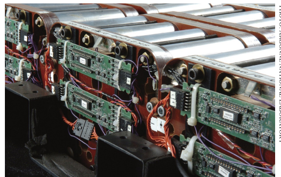
High-powered lithium batteries for use in hybrid electric vehicles. To meet BLUE Map targets, electric and plug-in hybrid electric vehicles would need to increase market share.
